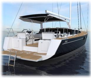
New fixed helm's seats with cockpit galley under seats A sink with small storage underneath to port A gas plancha with small storage underneath to starboard
