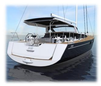
New large foldable aft transom  $(3,20 \text{ m} \times 0,80 \text{ m} / 12'6" \times 2'7")$ Convenient for easy bathing (high quality ladder with handrails) or farniente
